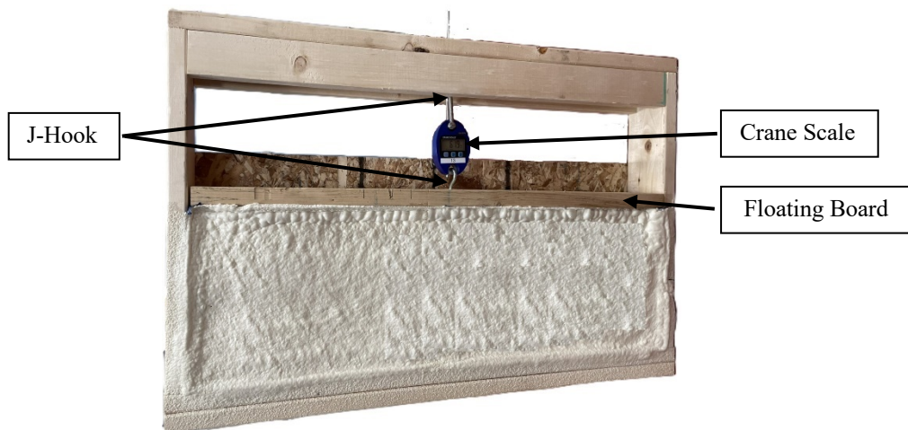
Picture 3. Large test jig after being sprayed
