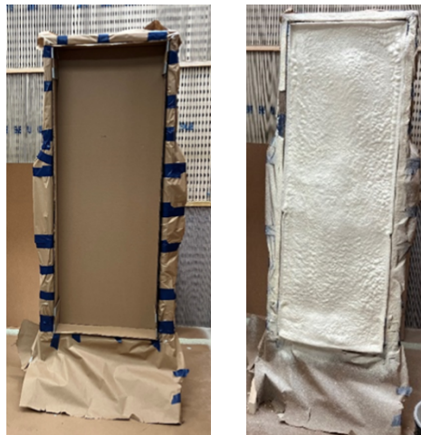
Picture 6. Cardboard box sprayed for physical testing
