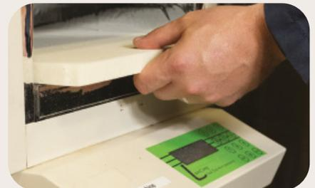
We perform extensive foam thermal conductivity testing, including testing at cryogenic temperature.
