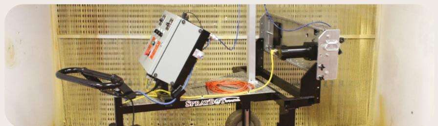
Our robotic machine can be used to ensure consistency and repeatability in spray test sample preparation.
